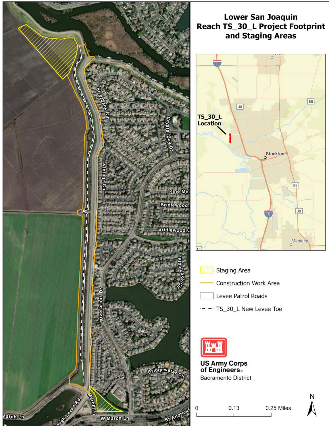
Figure 2. Reach TS30L proposed footprint, including staging area locations, construction work area, new levee toe location and levee patrol roads.
