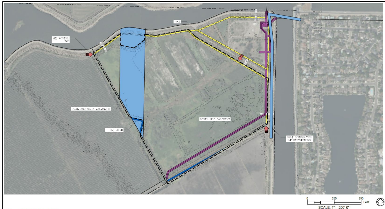
Figure 12. Existing utilities infrastructure and easements at the Fourteenmile Slough Pump Station (Parcel C)
